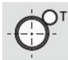
Figure 21. EEV Temperature Sensing Probe Installation
